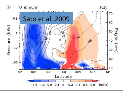
Latitudinal propagation of GWs The easterly jet in the summer hemisphere exhibits a slanted structure above 50 km in the mesosphere
