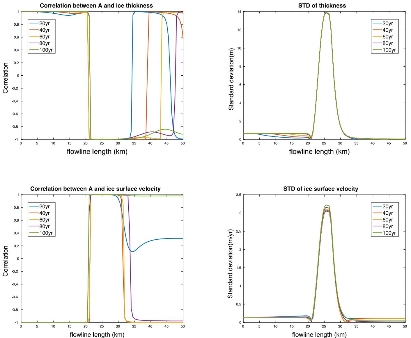
**Fig. 2.** Results of Experiment 1a, varying terrain height  $A$ . Shown are the correlation between  $A$  and ice thickness (upper left) and surface velocity  $u$  (lower left), and standard deviations of thickness (upper right) and velocity (lower right).
